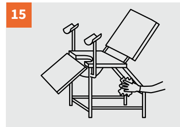
Clean the joints and the frame
