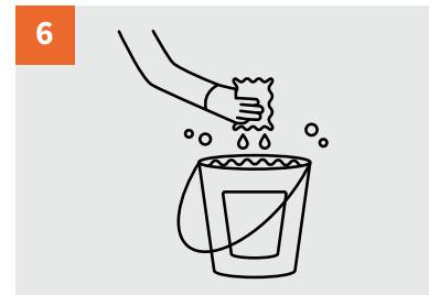
6 Dampen the cloth in a detergent solution
