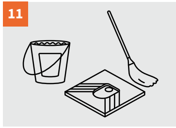
11 Using the detergent solution, mop around the outside of the squat toilet
