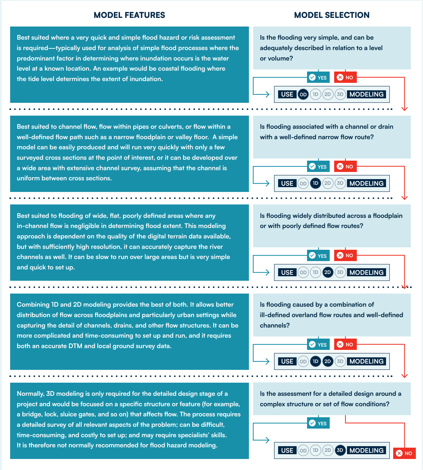
Figure 2.3 Decision Tree to Select Hydraulic Modeling Type for Flood Hazard Assessment
