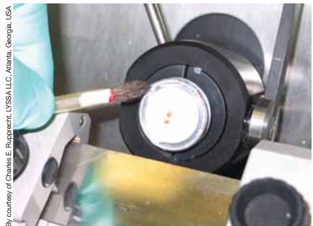
Fig. 15.13. Advancing the specimen through the cryostat blade while teasing the sections from the frozen block to position the section onto the microscope slide
