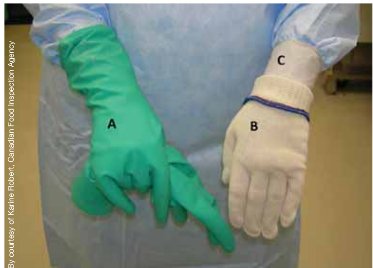
Fig. 3.2. Protective gloves recommended for necropsy areas: (A) heavy rubber glove, (B) cut-resistant glove, (C) laboratory glove
