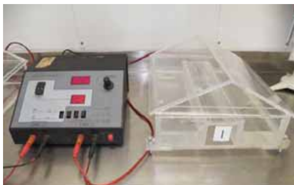
Fig. 26.3. Power supply and electrophoresis chamber, with lateral channels and a central support for glass slides
