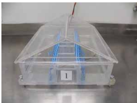
Fig. 26.4. Electrophoresis chamber, with the glass slides and connecting wicks made of viscose fabric for cleaning use (such as Perfex)
