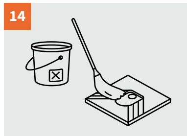
Repeat the process with chlorine-based disinfectant solution
