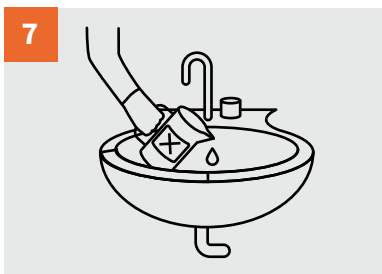
7 Pour a small amount of chlorine-based disinfectant solution into the plug hole and leave in contact without allowing solution to dry
