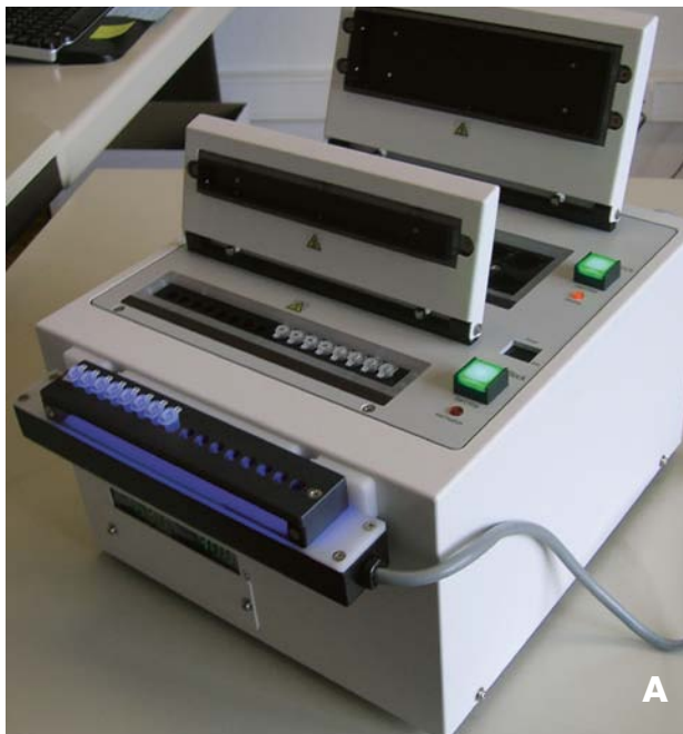
The Loopamp™ LF-160 incubator (A) used to perform the HAT LAMP reaction. After extraction of DNA, the LAMP reaction is kept at a constant temperature of 65°C for 40 minutes. The results are visualized under LED light (B). PC- Positive control, NC- Negative control. (Photo on the right is courtesy of E. Matovu)
