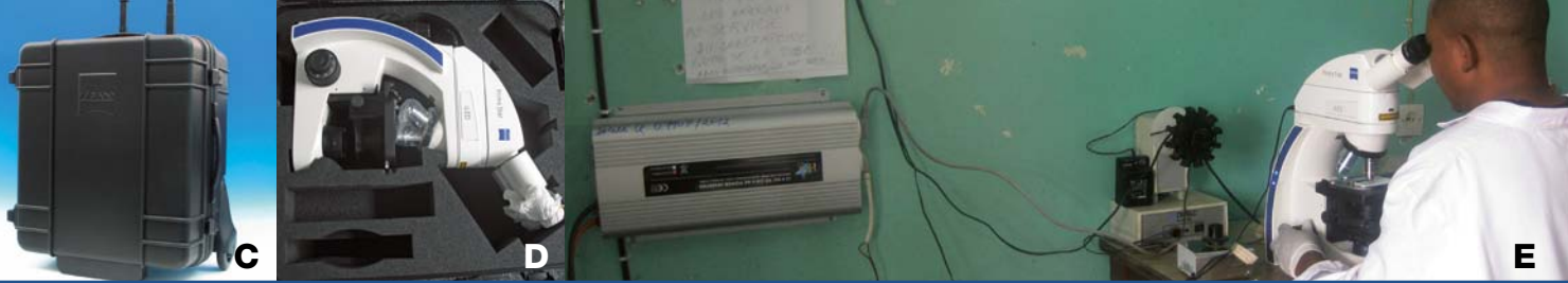
Carl Zeiss has developed a plastic box that enables easy and safe transportation of the microscope during active screening programmes (C&D). Panel E shows a technician operating an LED fluorescence microscope using solar energy in eastern Democratic Republic of the Congo. (Photos C&D are courtesy of Carl Zeiss AG)
