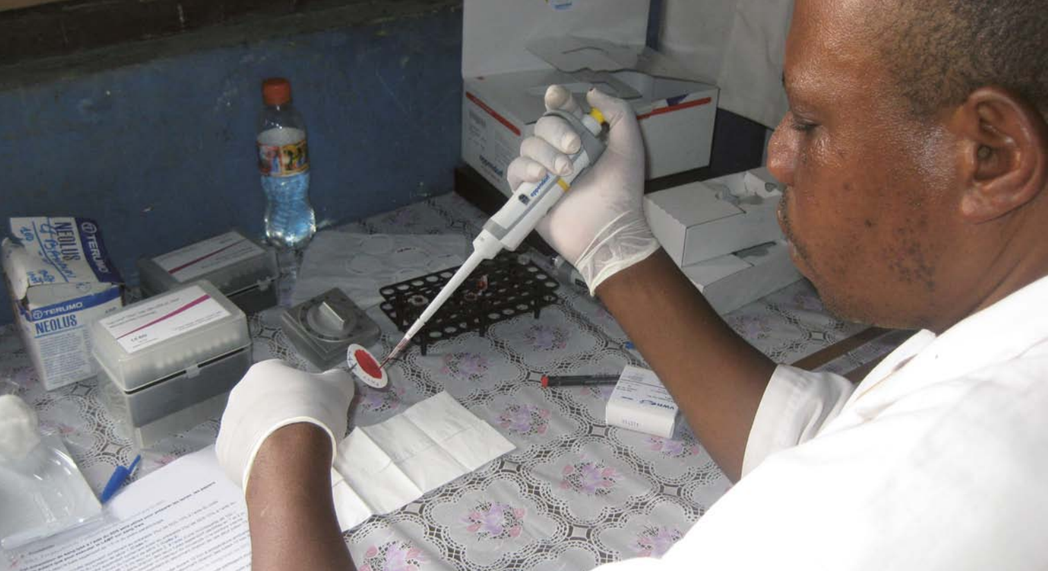
A technician applies blood from a participant on a filter paper at a rural health centre in the Democratic Republic of the Congo during clinical evaluation of LAMP for the diagnosis of HAT. The sample is left to dry at ambient temperature, then stored in a plastic pouch containing a desiccant, before being sent to a LAMP centre for testing.
