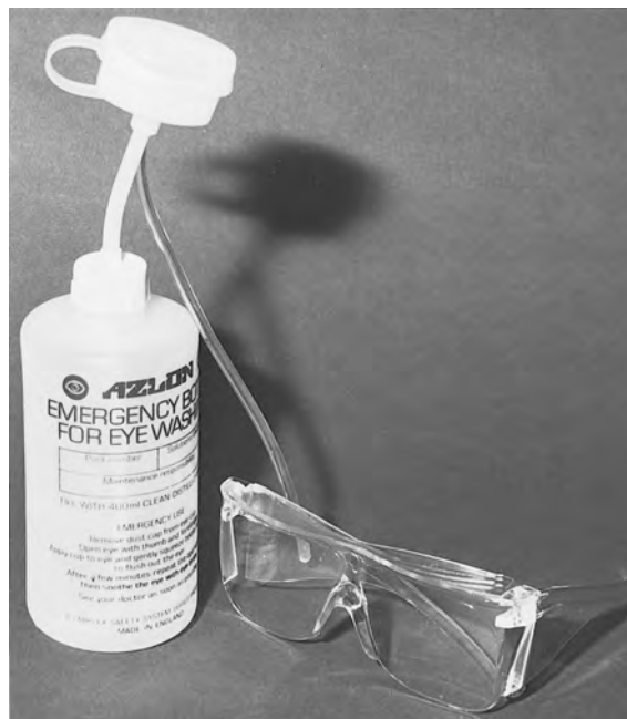
Plate 1.2 Left: 500mL emergency eye wash bottle. Squeezing the bottle gently sprays the eye. The waste liquid flows through a tube to the sink or collecting vessel. Instructions for use are printed in green on the bottle. Right: Protective eyeshields with closed in sides. The goggles are made from polycarbonate.
