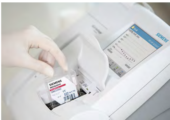
Plate 3.33 Inserting HbA1c reagent cartridge with sample into cartridge compartment. Courtesy Siemens Healthcare GmbH.
