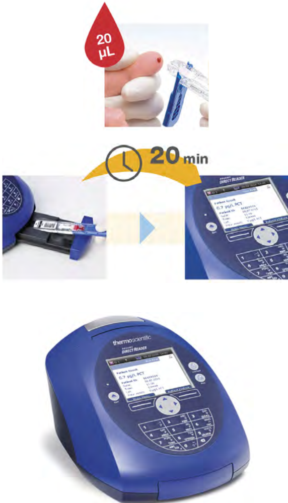
Plate 2.85 Upper: Summary of BRAHMS PCT direct test procedure. Courtesy of BRAHMS GmbH Thermo Fisher Scientific Inc. www.thermoscientific.com . procalcitonin Lower: B.R.A.H.M.S direct Reader' Copyright owner: B.R.A.H.M.S GmbH
