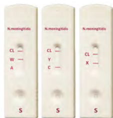
Plate 2.46 MeningoSpeed three cassette IC test to detect N. meningitidis serogroups: A, W, Y, C, X
