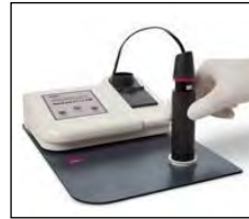
Plate 2.82 Quantitative measurement of CRP using Nycocard Reader 11. Courtesy of Axis-Shield. Available from www.alere.com
