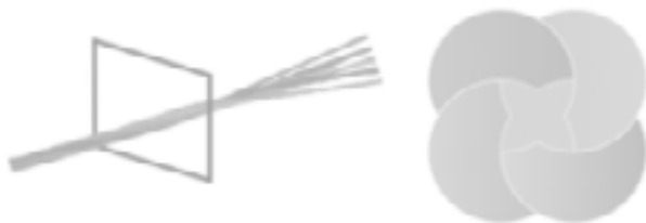
Figure 4. A transversal cut of a 5-thread rope.
