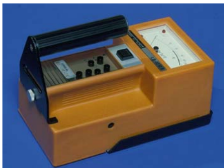
Figure A8.7. An example of beta and X-ray contamination monitor. Photo: HPA.
