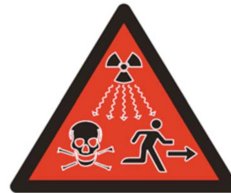
Figure E2b. Supplementary ionising radiation warning symbol. The symbol is intended for IAEA Category 1,2 and 3 sources defined as dangerous sources capable of death or serious injury. To be placed on the device housing the source, as a warning not to dismantle the device or to get any closer.
