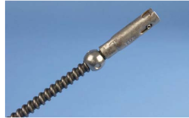
Figure E5. Very dangerous source from radiography camera (should never be picked up). Photo: HPA.
