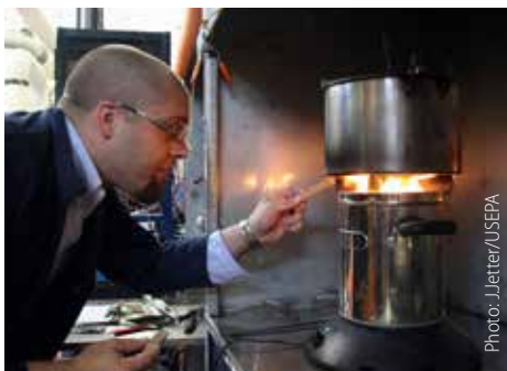
(a) testing emissions from a Philips fan stove at the US Environmental Protection Agency (USEPA) laboratory.
