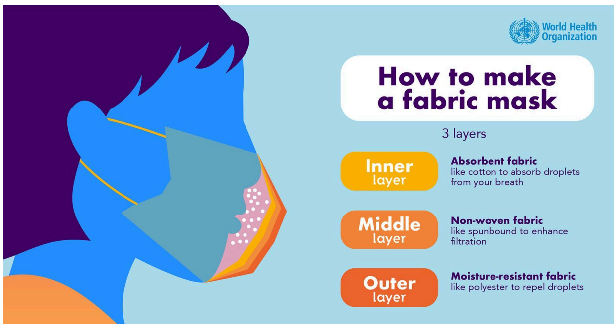
Figure 1. Non-medical mask construction using breathable fabrics such as cotton, cotton blends, polyesters, nylon and polypropylene spunbond that are breathable may impart adequate filtration performance when layered. Single- or double-layer combinations of advanced materials may be used if they meet performance requirements [85]
