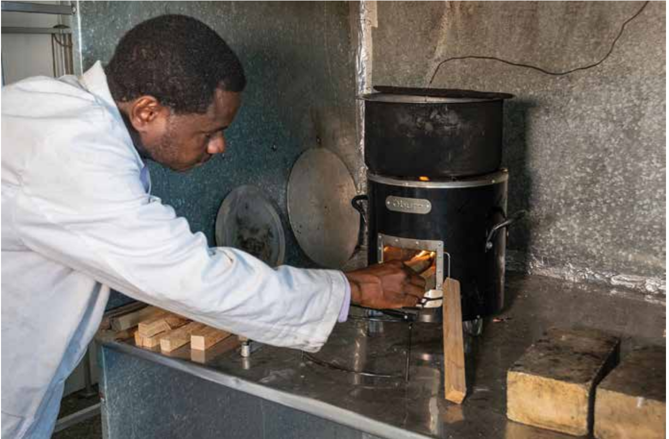
Testing a wood fuel cookstove in the laboratory at KIRDI, Nairobi.
