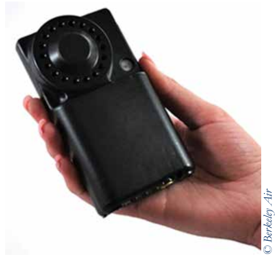
A PATS+ device, a lightweight, light scattering particle monitor with a battery life of up to 72 hours which can easily be worn.
