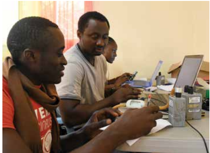
Calibrating the pump flow rate for a MicroPEM particle monitor, a small, easily worn device which includes both laser light scattering and gravimetric measurement systems.
