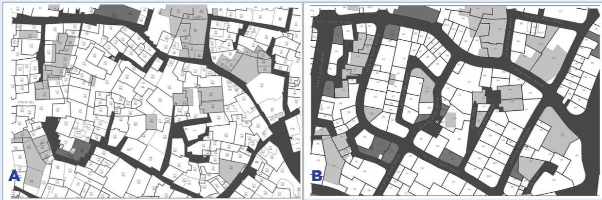
Figure 9: A block in Bhuj walled city A: Before land readjustment; B: After land readjustment Source: Environmental Planning Collaborative, Ahmedabad
