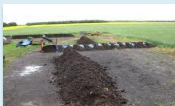
Aerated (Turned) Windrow Composting
