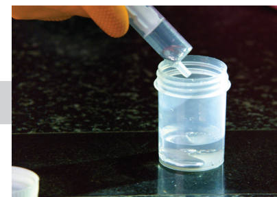
7 Transfer collected mercury into a container with water
