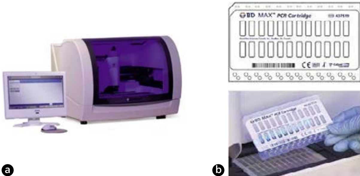
Fig. 2.1.5. Becton Dickinson equipment: (a) BD MAX™ System and (b) BD MAX PCR Cartridges
