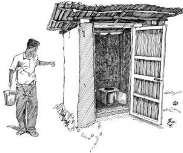
Bucket latrine showing bucket (Credit: Shaw, 2005)
