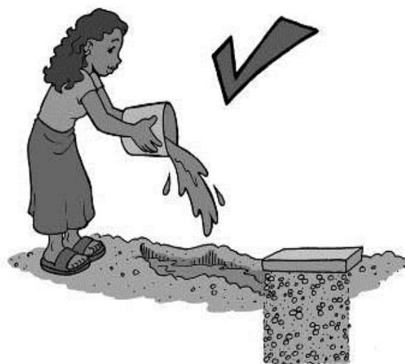
Wastewater going into soak pit
