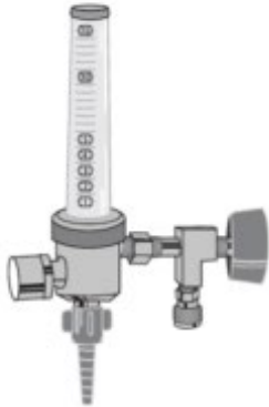
Thorpe tube (rotameter)
