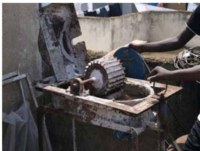
A pulping machine used to make sanitary pads from water hyacinth
