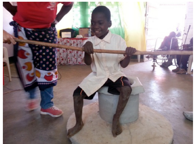
Sanitation for all. Inclusive sanitation technologies, such as raised latrines and grab rail, were tested to develop latrines for people with disabilities.
