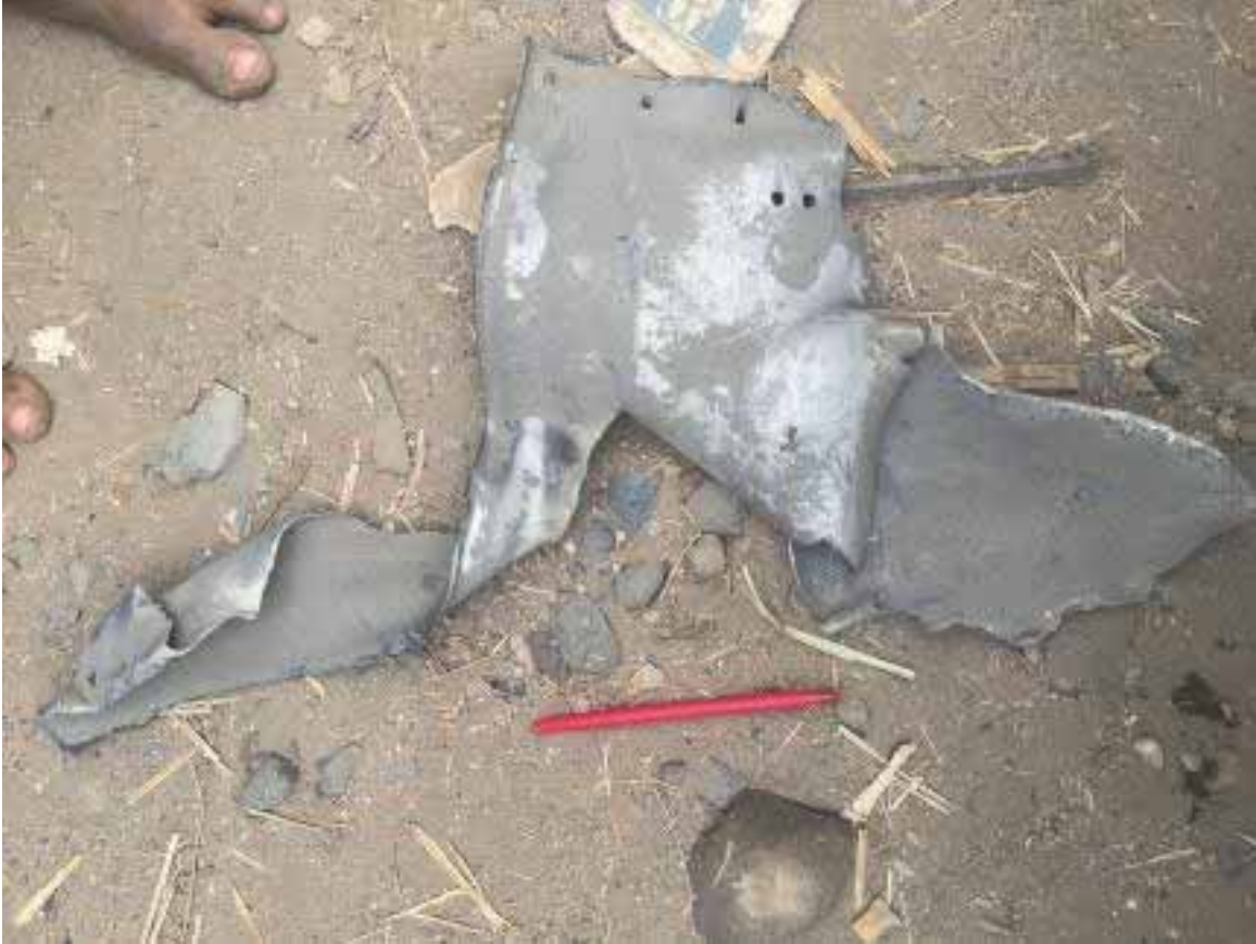
Remnant of a “strake,” part of a US-supplied JDAM satellite-guided bomb, found at the scene of the March 15, 2016 airstrike on Mastaba, in northern Yemen. © 2016 Human Rights Watch
