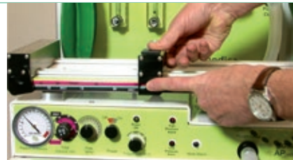
Patient pressure controlled by moving weights
