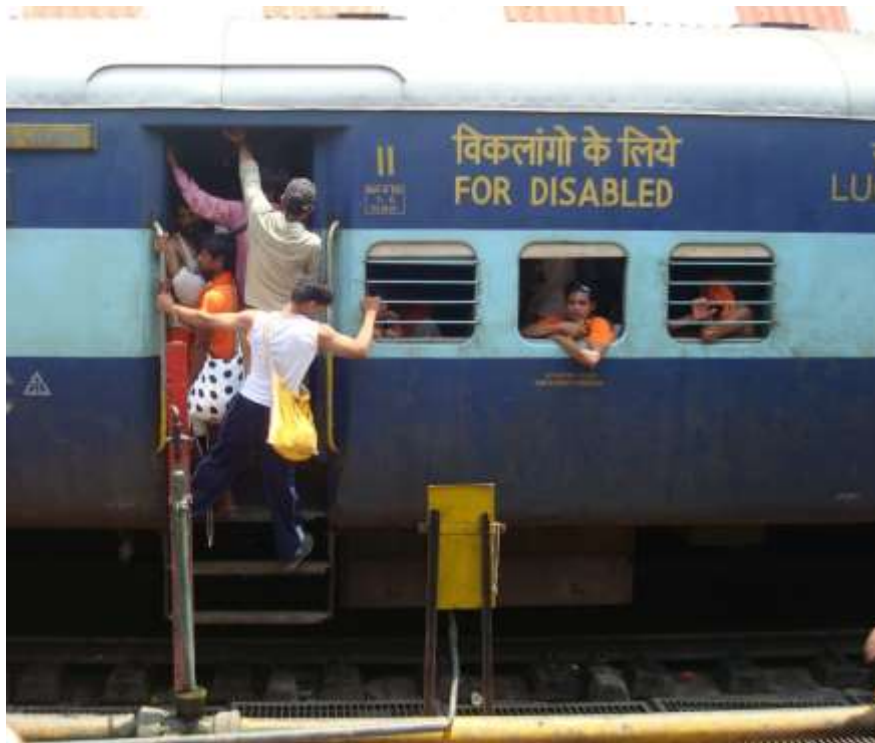
Figure 59: Train car for "Disabled" that is not accessible. Photo: Svayam/Jindal Saw Ltd.
