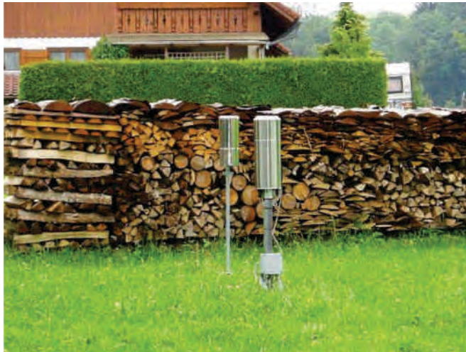
Figure 4.3: Real-time precipitation-station ( www.hnd.bayern.de )
