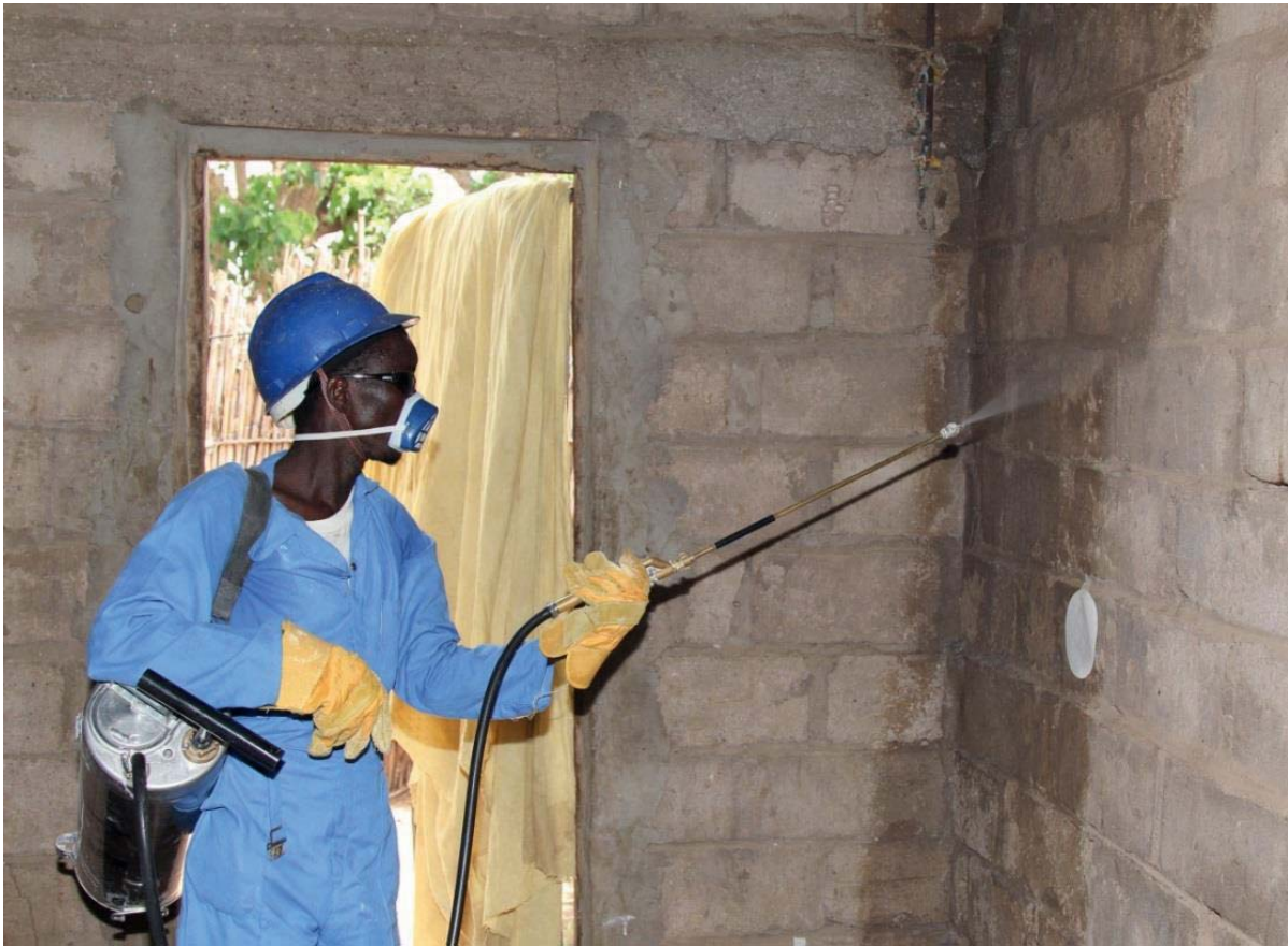
Fig. 33. Quality assurance of indoor residual spraying: filter paper on the wall is used to measure insecticide application (photo courtesy of S. Lindsay)
