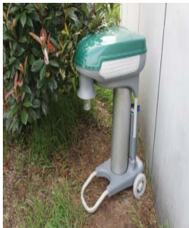
Figure 26. Sandfly CDC incandescent light trap © Shanghai Entry-Exit inspection and quarantine bureau, China.
