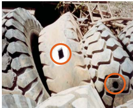
Figure 33. Holes cut in the tyres should be at 3, 6, 9 and 12 o'clock to prevent waterstagnation © Ashwani Kumar
