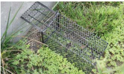
Figure 51. Conventional rat cage with conical entrance (also known as Wonder trap) © S. Senthil Nathan
