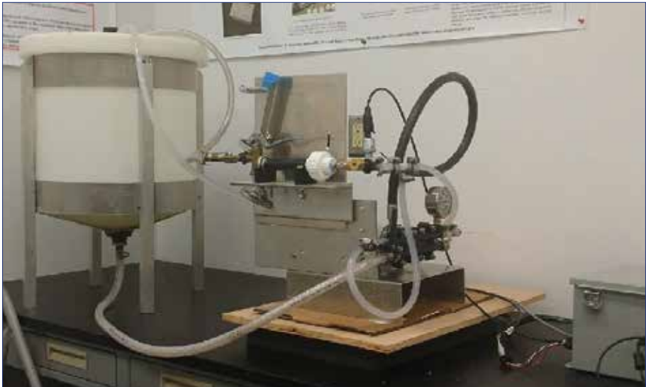
Figure 23. A software-controlled apparatus to test the abrasion resistance of the trigger valve (source: Navy Entomology Center of Excellence, FL, USA)
