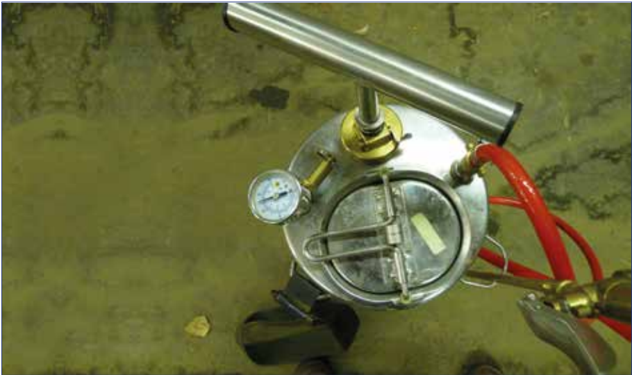
Figure 10. Air pump with handle for two hands and fitted with a locking device
