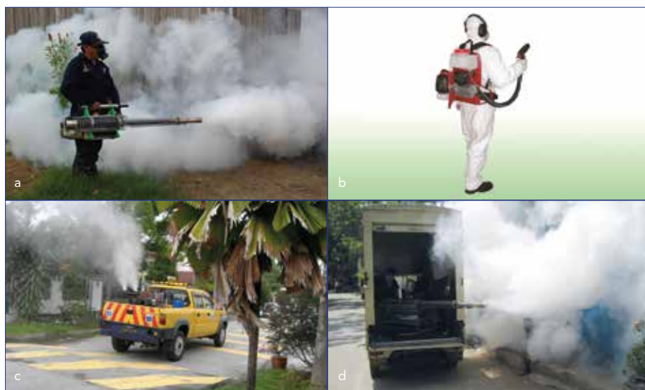
Figure 2. Space spraying against mosquitoes: examples of use of a (a) hand-held thermal fogger using an oil-based formulation; (b) knapsack cold fogger; (c) truck mounted cold fogger; and (d) vehicle-mounted thermal fogger
