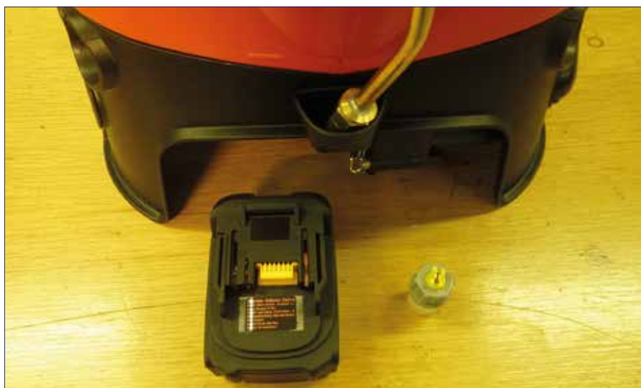
Figure 27. Sprayer showing battery in position in separate compartment below the spray tank
