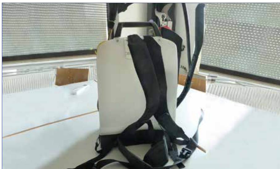
Figure 8. A lever-operated knapsack sprayer with shoulder and waist straps; these are required to minimize movement of the tank on the operator's body while pumping
