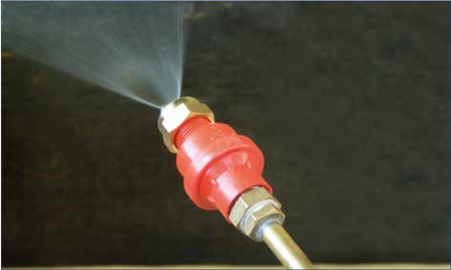
Figure 11. Example of a control flow valve (in red colour)
