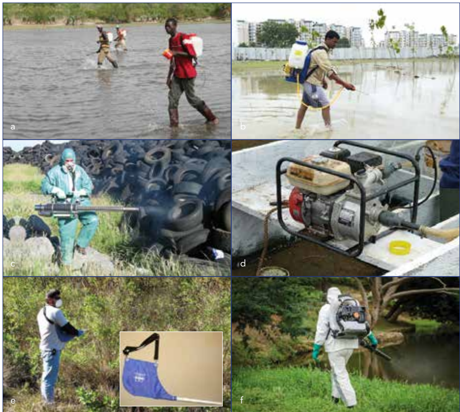
Figure 4. Examples of larvicidal application. Clockwise: (a) lever-operated knapsack, (b) motorized knapsack, (c) thermal fogger emitting large water-based droplets, (d) portable pump on a boat, (e) horn seeder granule applicator in vegetated areas, and (f) motorized mistblower adapted to apply insecticide granules to control mosquito larvae
