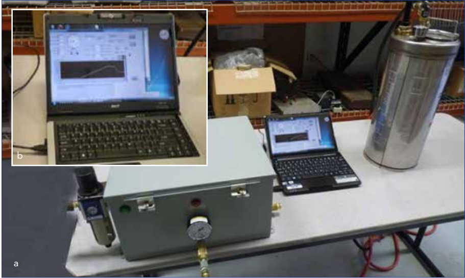
Figure 20. a. Testing tank fatigue of a compression sprayer using a computerized system (source: Navy Entomology Center of Excellence, FL, USA); b. Fatigue test monitored using a laptop
