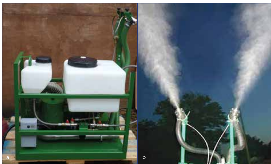
Figure 16. Vehicle-mounted cold fogger (a) and the cold fog being generated by it (b)
