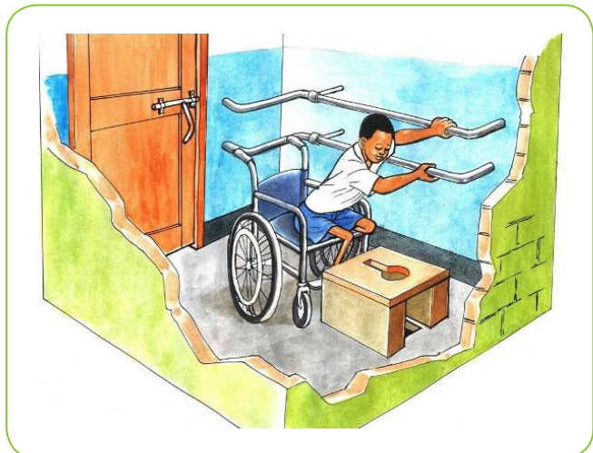
Figure 24: Toilet in Tanzania with toilet stool and grab rails (Source: Government of Tanzania)
