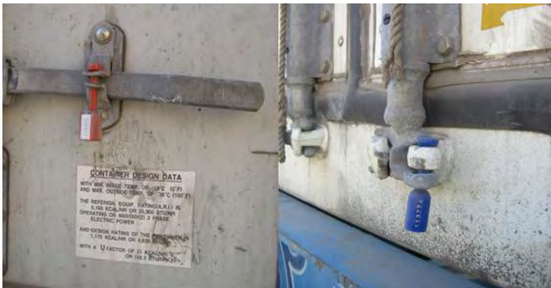
Figure 23.4 Sealing of ISO shipping container
