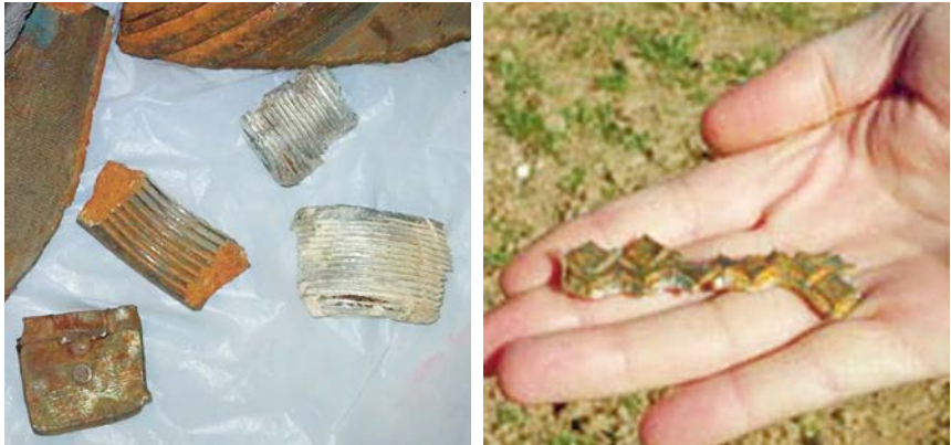
Figures 13 and 14. Natural fragmentation (left) from a mortar projectile recovered in Baghdad, Iraq in Jan 2006 (photo credit: Bryan G. /U.S. Army), and a section of pre-fragmented munition casing (right) (source: USDA, 2006, p. 20).
