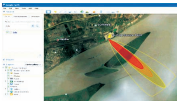
Figure 36: Damage and distance modeling using ALOHA and MARPLOT represented on Google earth.
