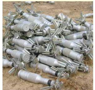
PICTURE 1.21 Various unexploded submunitions. Extremely unstable: BLU-97, DM1385, PTAB-2.5KO. UNMAS Photos/Thomas Enke
