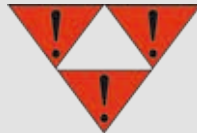
Must not be subjected to impact and must be protected against impact from other waggons (railway).
