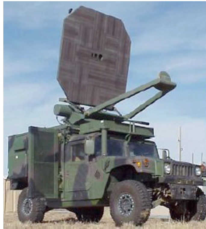
Active Denial System (ADS) mounted on top of a Humvee. Photo: US military
