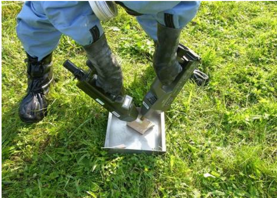
Figure 2.2: OPCW inspector using two detectors of different technologies to obtain a “confirmed” detection during training in the Czech Republic, 2008
