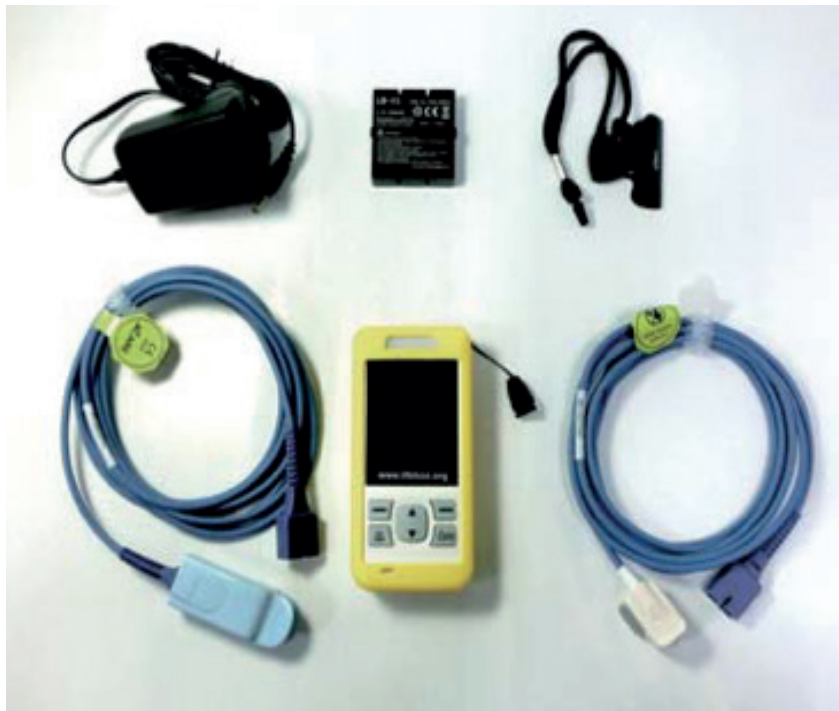
FIGURE A2.2 Lifebox pulse oximeter and accessories
