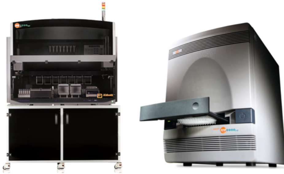
Figure 9. Abbott Molecular platforms for automated sample preparation ( m2000sp , left) and real-time PCR analysis ( m2000rt , right) for MTBC and first-line DST
