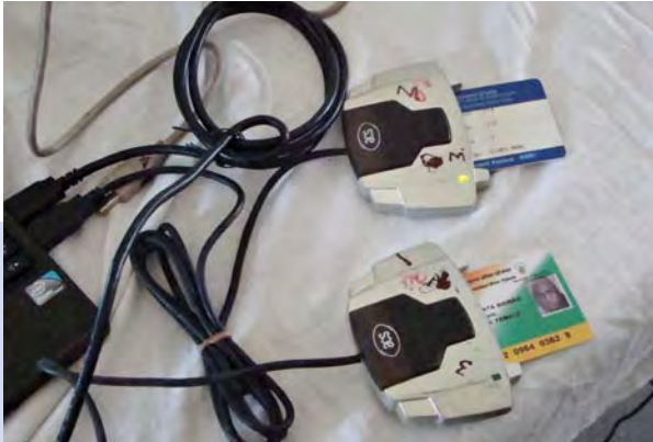
A Field Key Officer verifies that he has witnessed and approved enrolment by putting his FKO card into one reader while another reader records his verification on the Smart Card.
