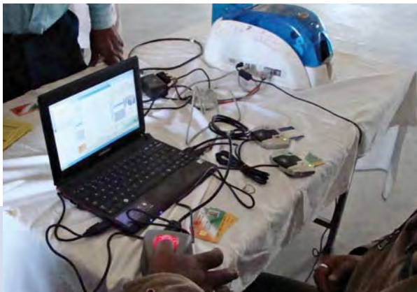
A laptop computer, RSBY software and peripherals provide everything needed for one-stop enrolment and distribution of Smart Cards.
