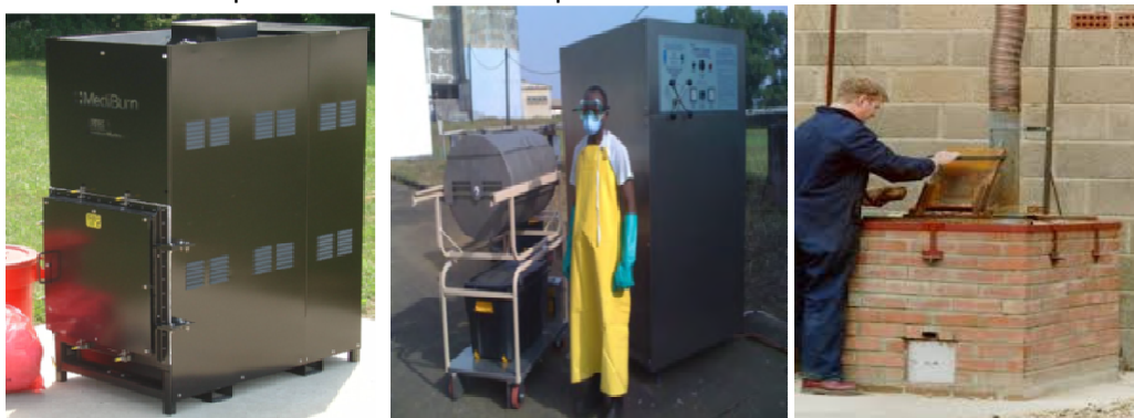
Figure 8: Pyrolytic Incinerator, Autoclave and De Montfort Incinerator for treatment of HCW
