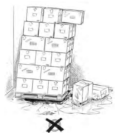
Figure 9. Tipping Pallet Due to Un-level Floor
