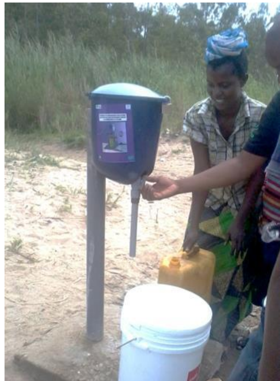
Figure 3: Chlorine Dispenser used in the DRC (Armitage, 2013)
