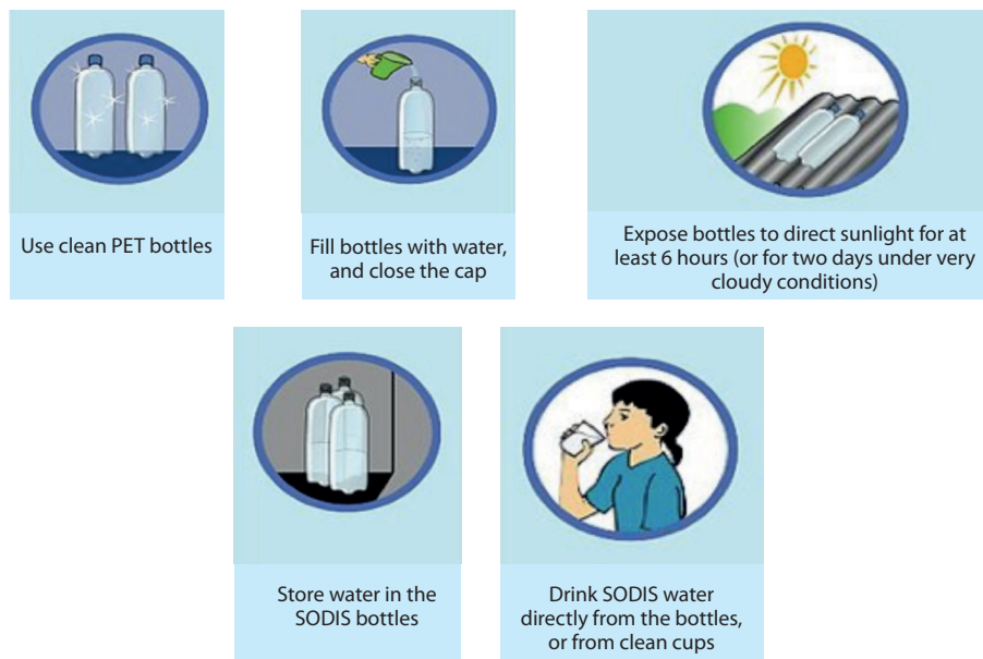
Fig.13 Practical Water Treatment Methods at household
