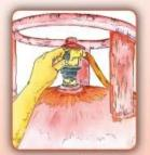
Switch off the gas supply from the cylinder regulator, after use.
