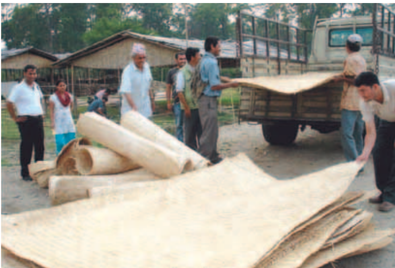
Photo10c: Bamboo mats as construction materials in Habitat for Humanity Houses © UN-HABITAT
