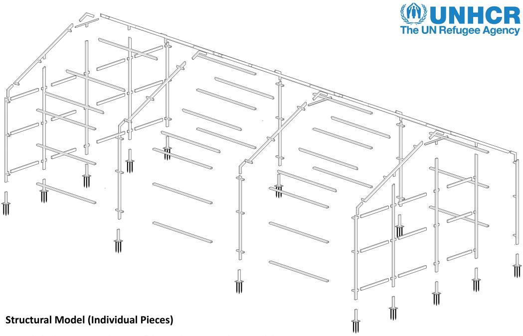
An exploded axonometric diagram of the steel structure, showing all the male and female pieces that make up the T-Shelter.
