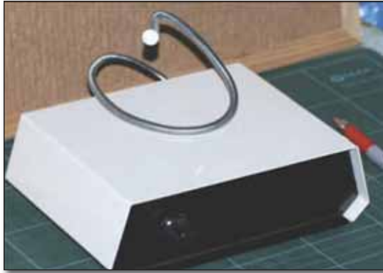
The LED light illustrated here can run for a minimum of 200 hours on four standard 1.5-volt batteries.
