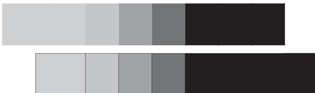
Fig B-2. Simulation of two test exposures obtained with a stepwedge
