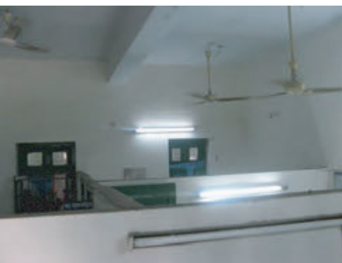
High ceiling (4.15 m), open partitions, ceiling fans for dilution of room-air, fanlights above window and door for cross ventilation
