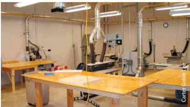
Figure 7 Example of a workshop for vocational training with proper safety ventilation
