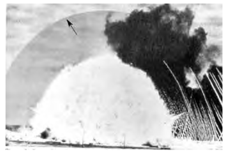
Figure A.5 Explosive detonation. Note the blast front indicated by the arrow. 7
