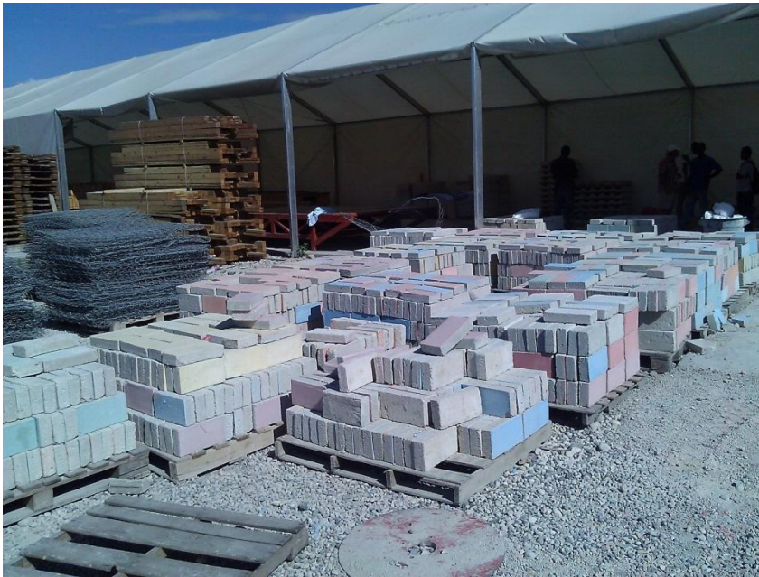
IFRC paving slabs made from reprocessed rubble
